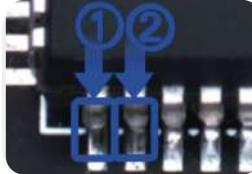
Cold solder can be quickly detected with the AI pin algorithm and unaffected by lack shadow showed on the image
