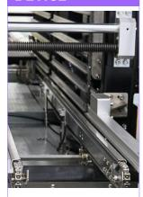
Two parallel chains at the side exit with a pusher device on each chain.
