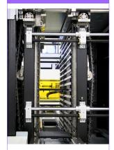
The limit photoelectric sensor detects the correct PCB position.
