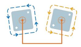
Vantage Series dual-head, dual-valve with patented\* real-time correction in the x and y-axis automatically adjusts to dispense to skewed parts avoiding impact to yield.
