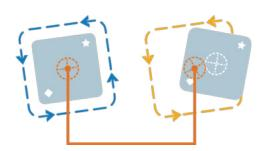
Early fixed-pitch, dual-valve designs could not adjust for individual part-to-part skew, negatively impacting yield.
