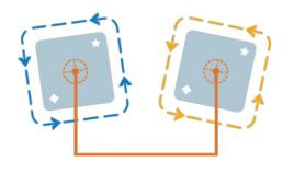
Forte MAX dual-valve with patented\* real-time correction automatically adjusts for individual part skew and height variation in the x, y, and z-axis to avoid impact to yield.
