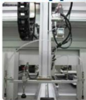
Pick-and-place method: single-head pick-and-place mechanism
