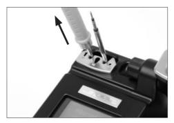
Pull slightly to remove the cartridge
