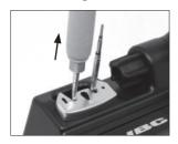
Place the handpiece in the extractor and pull to remove the cartridge.
