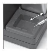
**Wiping:**Use the slots to remove remaining particles.
