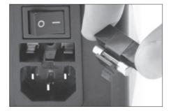
2. Insert the new fuse into the fuse holder and return it to the station.
