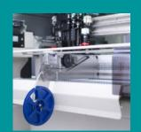
Intelligent feeders in all common sizes. Component spectrum from 01005 to 100x150 mm, component height up to 15mm
