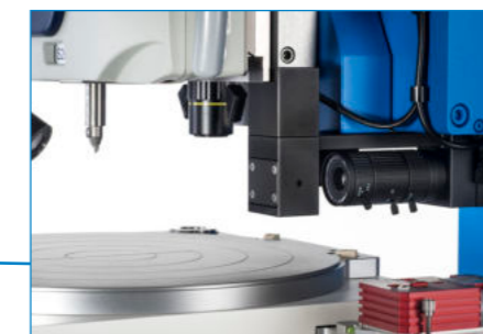
Integrated image capture and side alignment cameras
